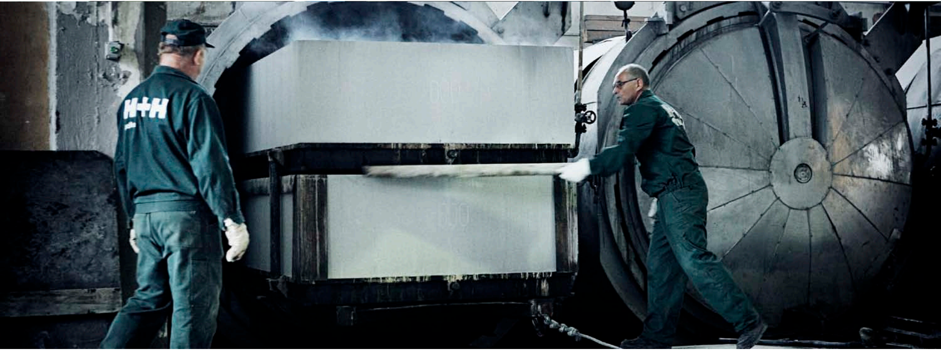
Coming out of the autoclave the aircrete products are cooled and are packed ready for transport.
